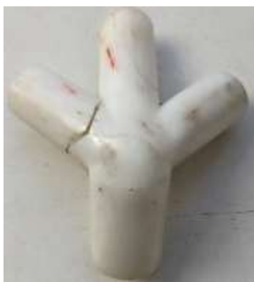
Fig. 1. Example of a problematic part for frame connections
